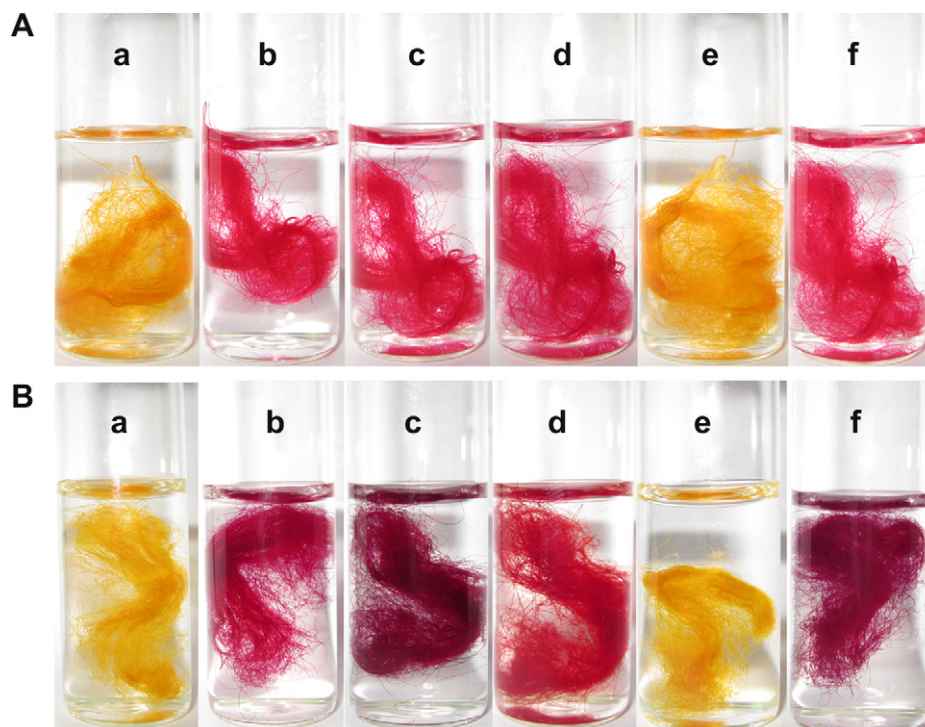
Fig. 10. The color-changing properties of P-PAN TASF in aqueous solution after (a) 0 s, (b) 1 s, (c) 20 s, (d) 24 h, (e) neutralization, and (f) next cycle 20 s. (A) 4 M HCl, (B) 4 M NaOH.
