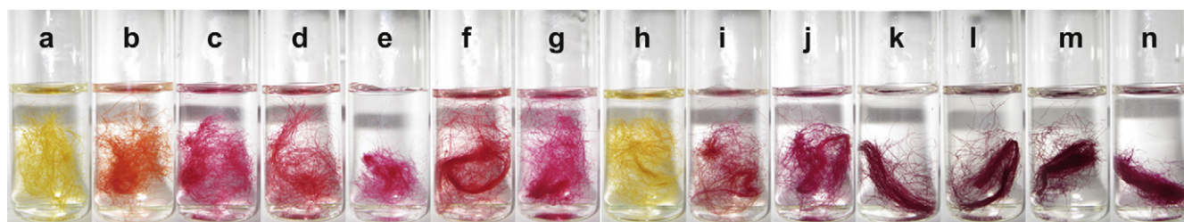
Fig. 11. The color-changing properties of P-PAN TASF in (a) CH 3 COOH, 4 M, (b) citric acid, 4 M, (c) H 3 PO 4 , 4 M, (d) HNO 3 , 4 M, (e) HCl, 4 M, (f) HBr, 4 M, and (g) H 2 SO 4 , 4 M. (h) Na 2 CO 3 , saturated aqueous solution, (i) Ca(OH) 2 , saturated aqueous solution, (j) Na 3 PO 4 , saturated aqueous solution, (k) Ba(OH) 2 , saturated aqueous solution, (l) Na 2 SiO 3 , saturated aqueous solution, (m) KOH, 4 M, and (n) NaOH, 4 M.
